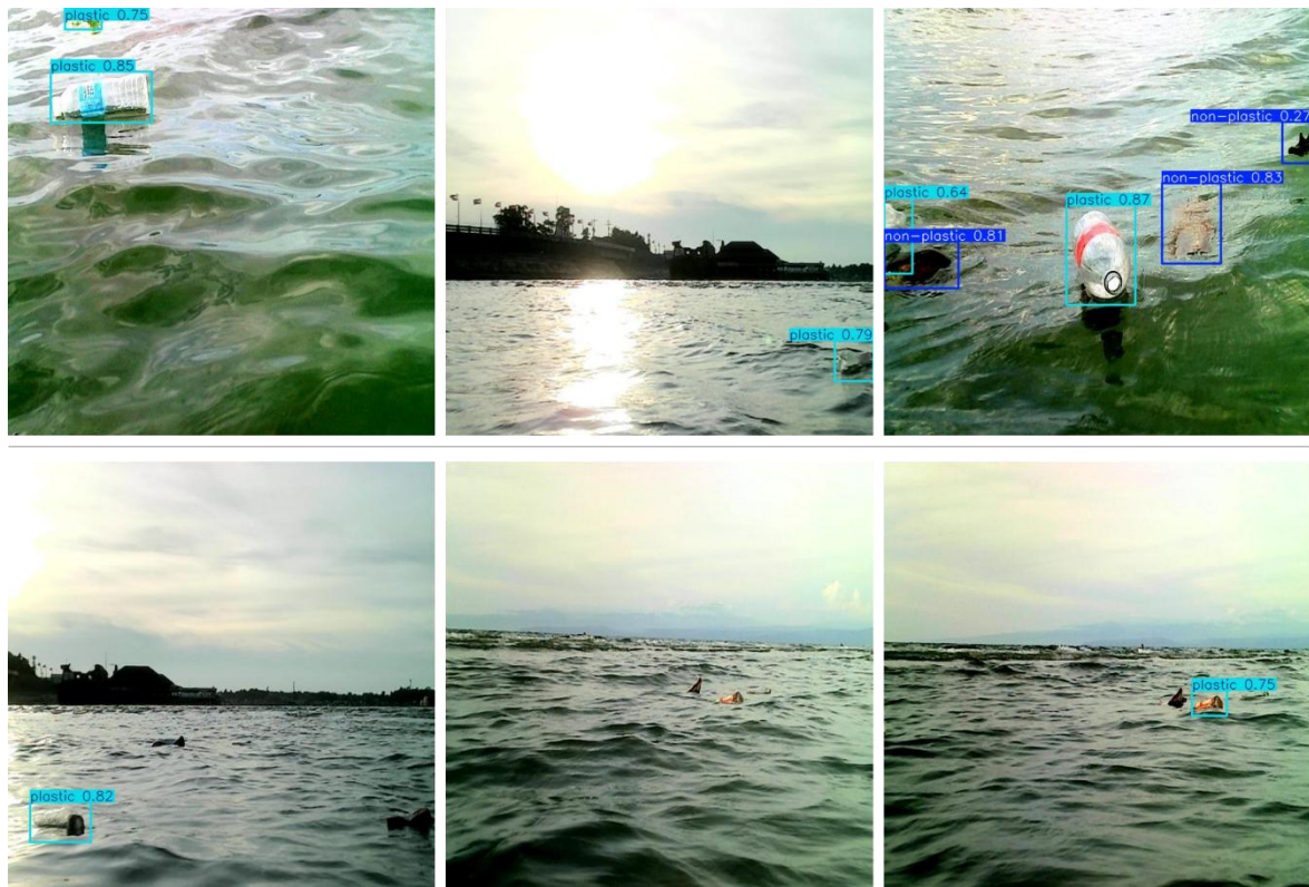
Figure 5. Qualitative results of the proposed YOLO11n with CBAM model. The top row illustrates detection results under challenging environmental conditions, including irregular object shapes, dynamic water surfaces, reflections, and varying lighting. The bottom row presents representative failure cases, including missed detections caused by difficulties in detecting small or low-contrast objects
