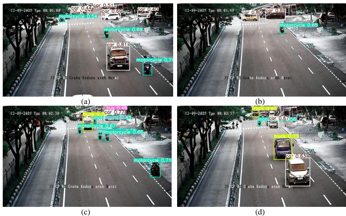
Figure 2. The result of vehicle detection using YOLOv5
